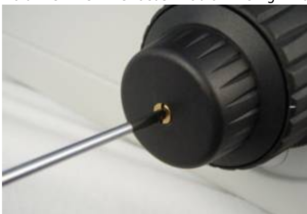
Use a flat head screwdriver to remove the inner brass screw.
