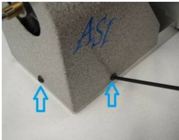
Install cover with screws as shown
