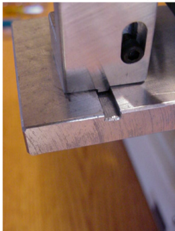
Figure 6: Tab on adjustment bar slides into groove on baseplate
