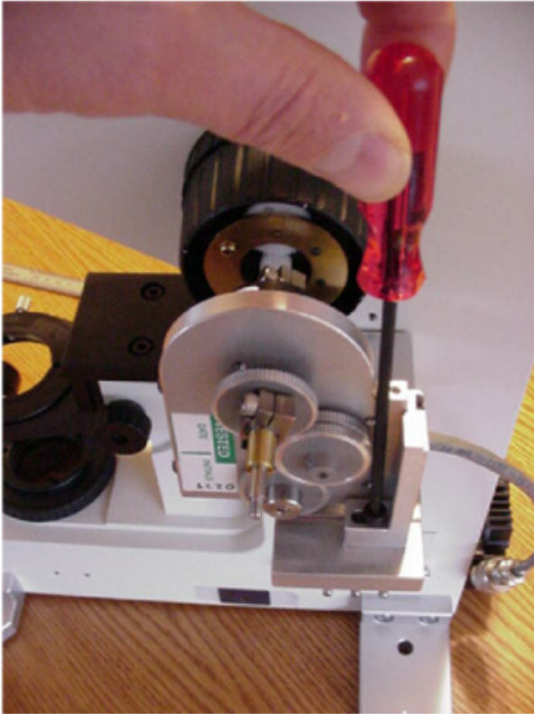
Figure 7: Secure, but Do Not tighten , horizontal adjustment screw to hold drive in
