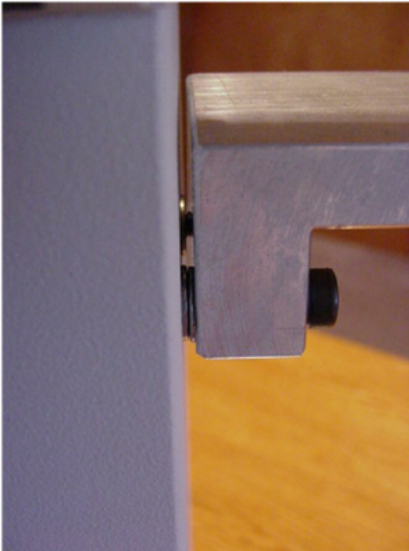
Figure 4c On some early drives two washers were used to position the drive out.
