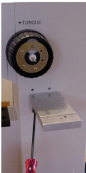
Figure 4a Installing baseplate
