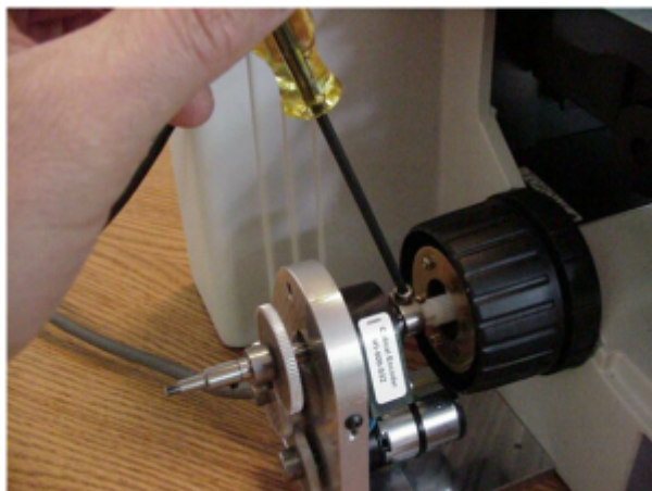
Figure 10: Tightening the drive shaft clamp
