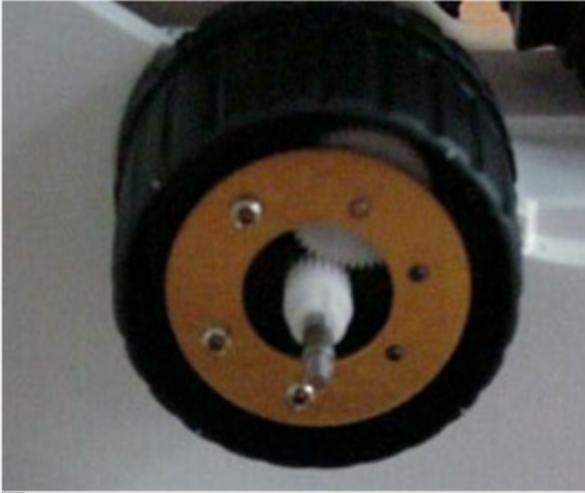
Figure 3: Pull knob straight off to expose shaft
