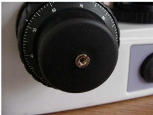
Figure 2: Use screwdriver to remove nut
