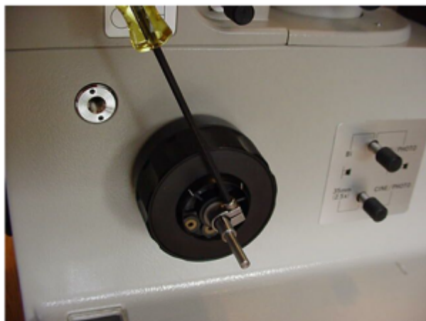
Figure 3c. Use 7/64" Allen securely tighten clamp
