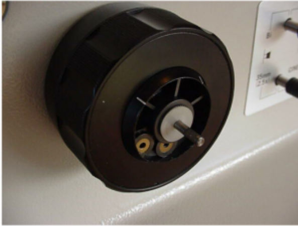
Figure 1.b Pull Knob off to Remove Fine Focus Knob
