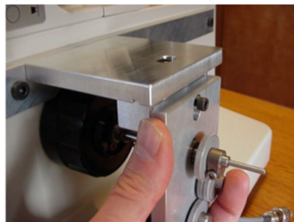
Figure 4b. Slip drive into groves and hold in place while screwing in vertical adjustment screw.
