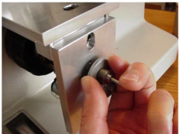
Figure 4e. Check for slippage by holding onto Drive shaft gear while turning the left fine focus Knob on the microscope.
