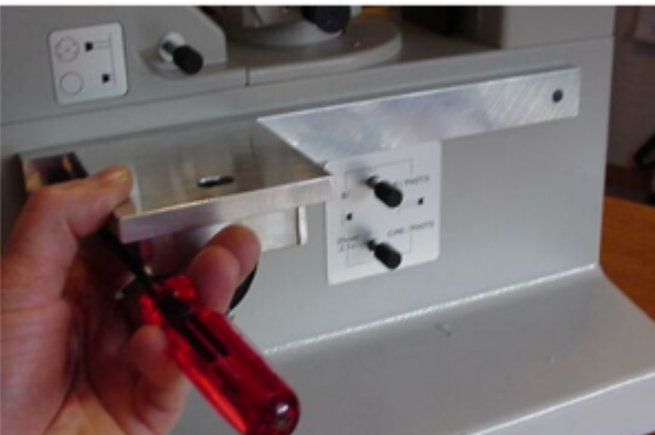
Figure 2b. Attach side plate to microscope with 5mm screws
