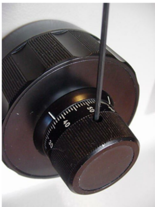
Figure 1a. Use 1.5 Allen to Loosen set screw
