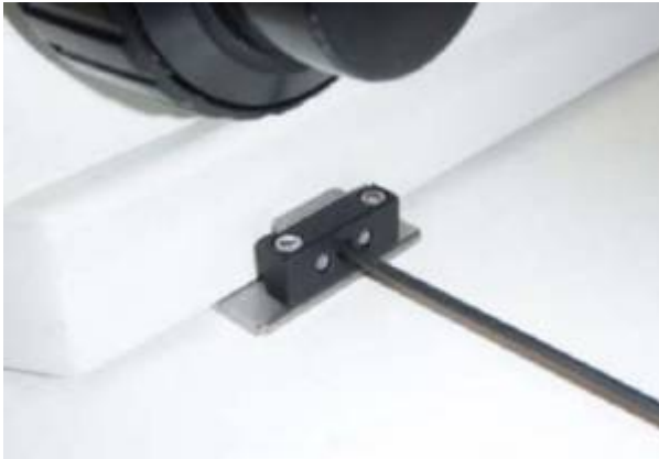
Figure 10: Tighten base plate clamp after drive is installed & roughly aligned
