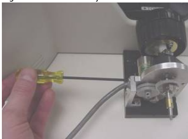
Figure 10: Vertical Adjustment screws
