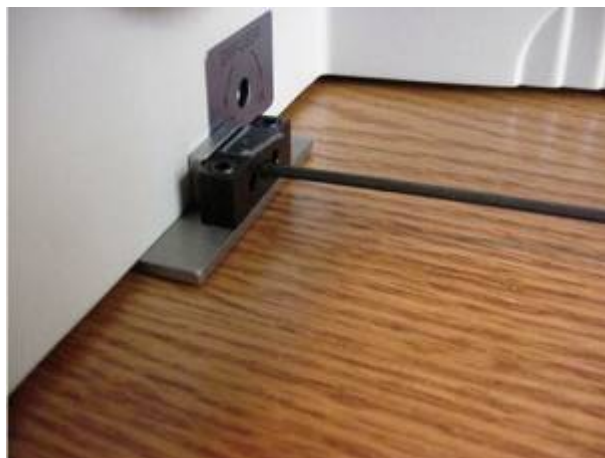
Figure 11: Tighten Baseplate set screw
