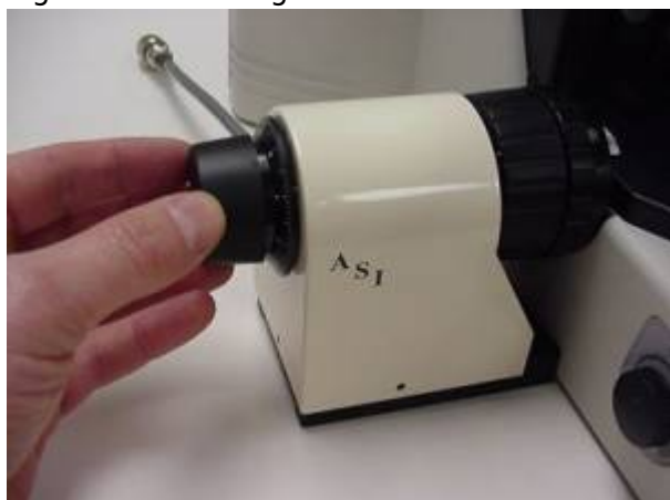
Figure 13: Installing cover and focus knob
