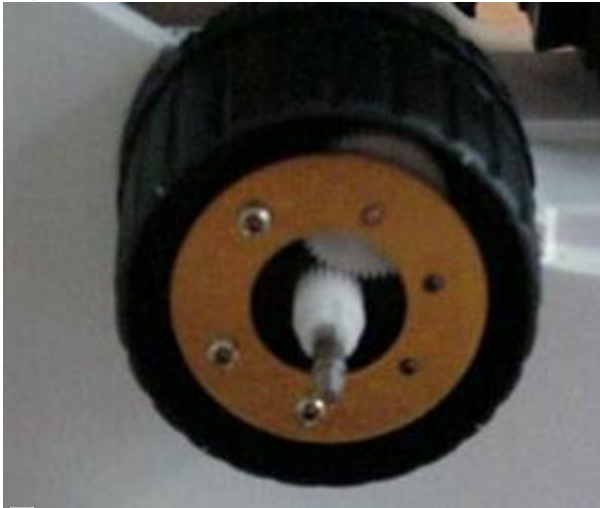
Figure 3: Pull knob straight off to expose shaft – Do not twist.
