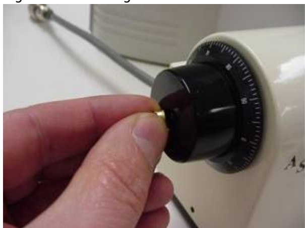
Figure 14: Installing cover and focus knob
