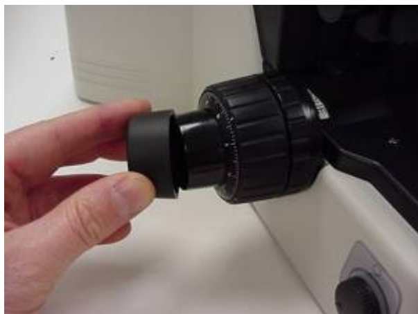
Figure 1: Pull off rubber boot
