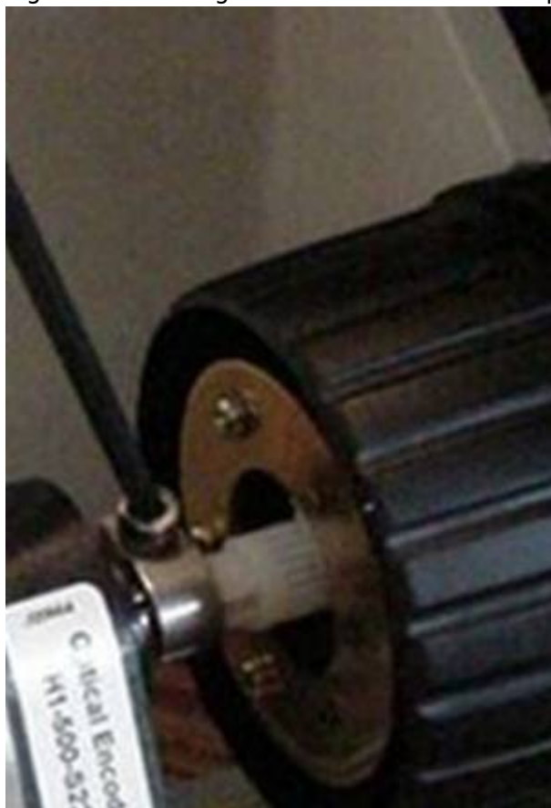
Figure 8: Tightening drive shaft clamp
