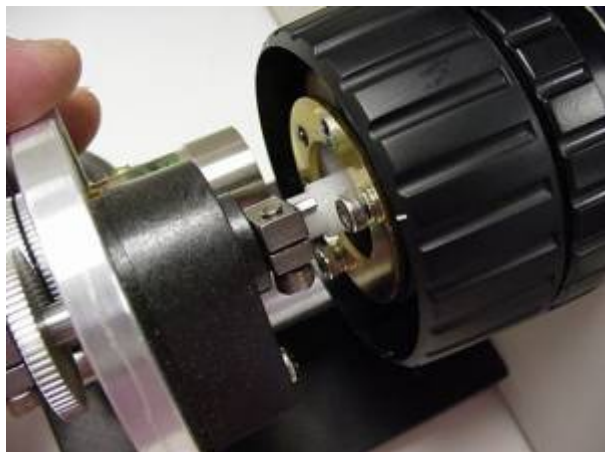
Figure 7: Installing Z-drive. Note tab on clamp slides into notch on plastic gear
