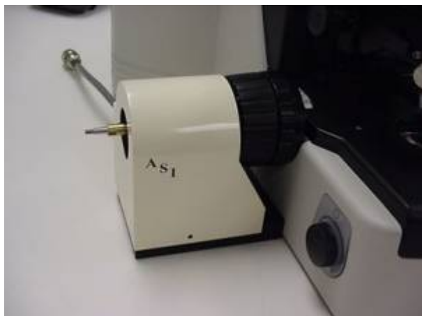
Figure 12: Installing cover and focus knob
