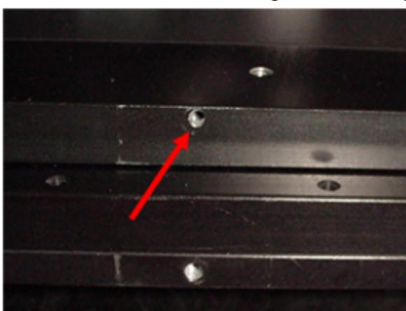
Insert's setscrew access on rear of stage.
