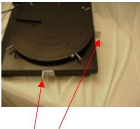
Location of two shipping brackets to remove before use.
