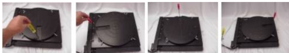
Four screws are used to attach wafer holder
