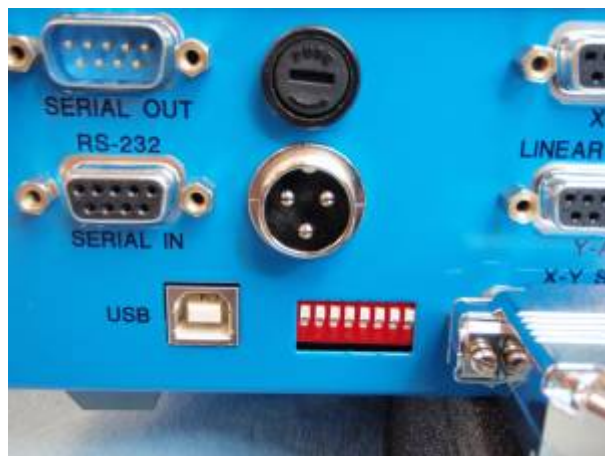
Figure 23. Power Connector on MS2000
