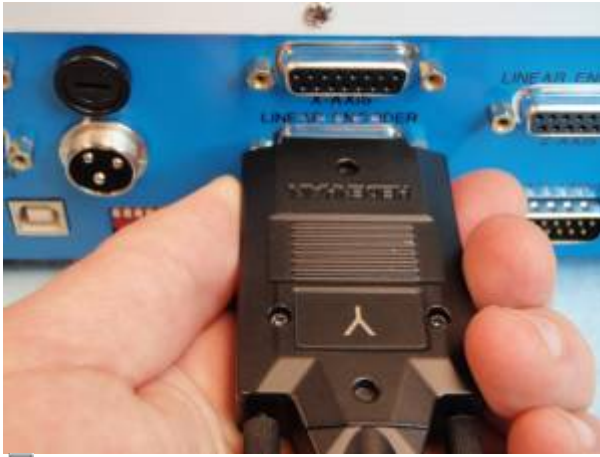
Figure 11. Y Axis Linear Encoder plugged into controller. (bottom plug).
