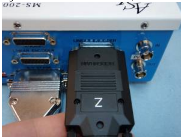
Figure 18. Z-Axis Linear Encoder plugged into controller
