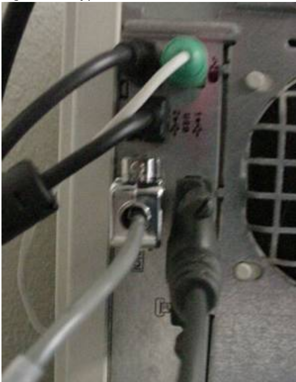
Figure 22. Serial cable connected
