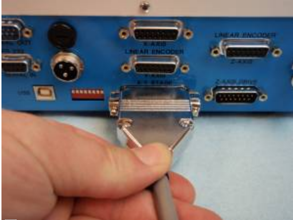
Figures 8. XY Stage cable plugged into controller
