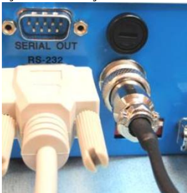
Figure 20 Serial-connected on to MS-2000
