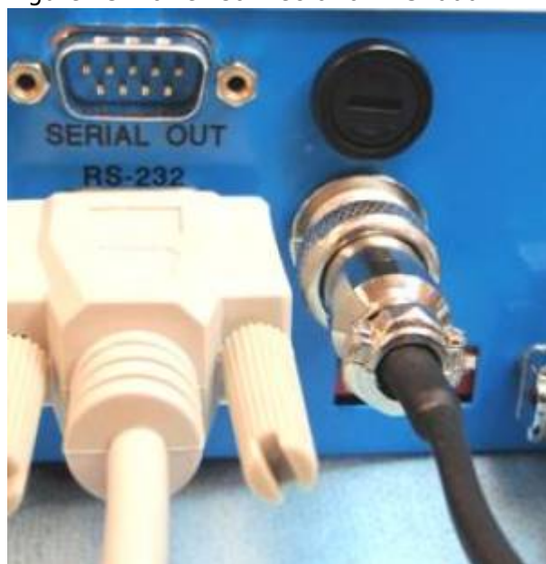
Figure 24. Power Plug connected to MS2000
