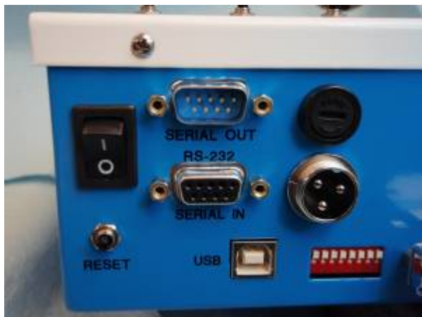
Figure 19 Serial-In Plug on MS-2000
