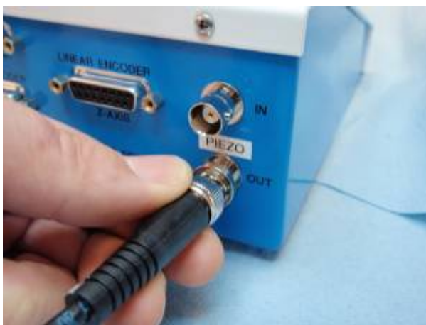
Figure 25 Piezo Out Plug on MS-2000
