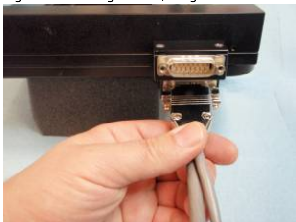
Figure 4. X-axis cable connects to bottom stage plug.
