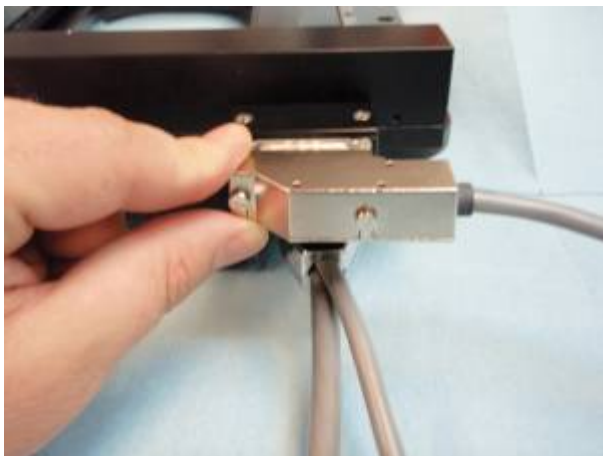
Figure 5. Y-axis cable connects to top stage plug
