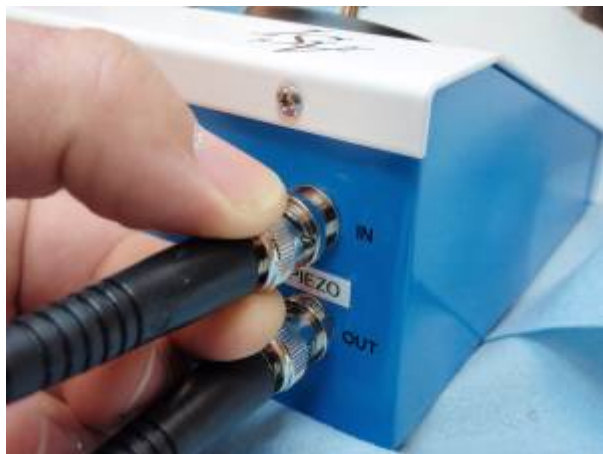
Figure 26 TTL-In Plug on MS-2000
