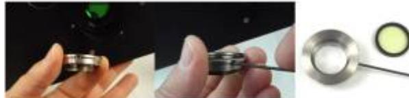
With the filter inside or out of the C-Mount, thread the C-Mount onto the camera till it is tight.
