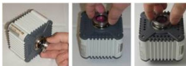
Next, add the camera and C-Mount combination onto the Filter Wheel with a 2mm driver. The small filter retaining set screw should not interfere with the outer set screws.
