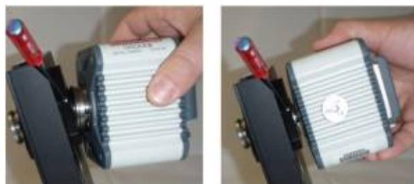
Tighten the three retaining set screws. They are 120 degrees apart from each other.
