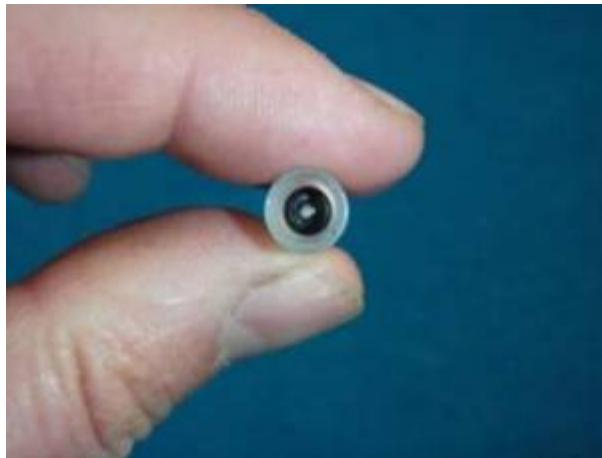
In order to get a good seal the pipette glass must go through the o-ring that is in the 2nd part of the pipette holder. The 2nd part of the pipette holder is tightened to compress the o-ring to make a seal around the glass pipette.
