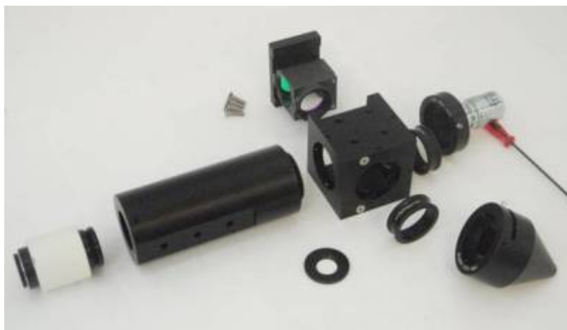
Figure 2: Exploded view of a MIM configured for epi-fluorescent illumination.
