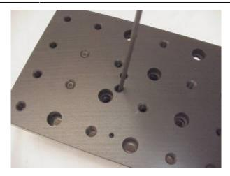
The LS-50 has less travel than the LS-100, so to access the counter-bores on the connector end of the stage, it is necessary to remove the connector housing. This is accomplished by removing the jackscrews on the connector, removing the connector cover, and removing the connector housing screws. Carefully move the connector and wiring out of the way while attaching the top plate screws. Reinstall the connector when completed.
