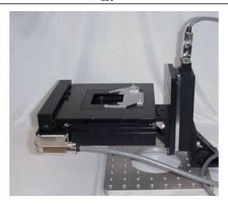
The photos above show a pair of LS stages set up for XY motion, and an ASI stage mounted to an LS-50 Z-axis unit. The LS-50 could also be mounted directly below the ASI stage as shown below, where the LS-50 is extended to its maximum travel.
