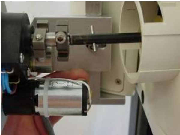
Figure 7: Slide ASI drive shaft over zoom shaft
