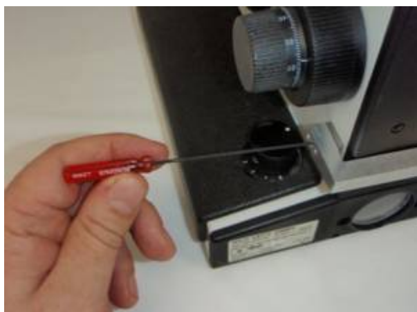
Figure 2c: Use 1.5mm Allen to tighten adjustment bar
