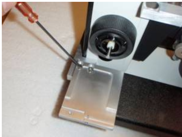
Figure 2d: Use 2mm Allen to loosen baseplate screws
