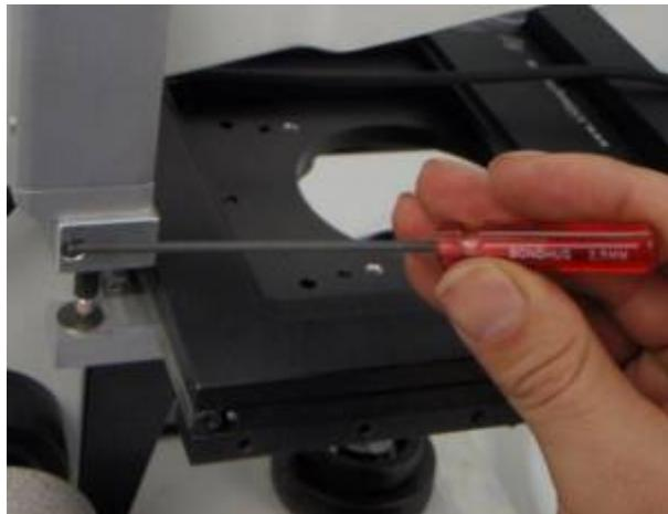
Bring the stage up to the correct focal position for the common objectives used. Position the encoder & encoder clamp so that the ball on the end of the encoder's plunger mates with the round carbide plunger stop. Insert the encoder into the encoder holder & slide the encoder down until there is about 1 to 3 millimeters worth of upward travel left on the encoder's plunger. Hold the encoder in place & use the 2.5mm Allen wrench to tighten the screw to secure the encoder in place.
