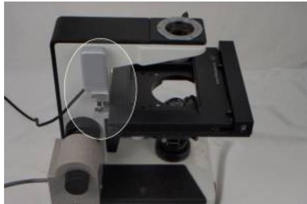
This completes the installation and alignment of the ASI linear encoder onto the Leica / Leitz LABORLUX S series microscope. Please refer to your ASI manual for further instruction.
