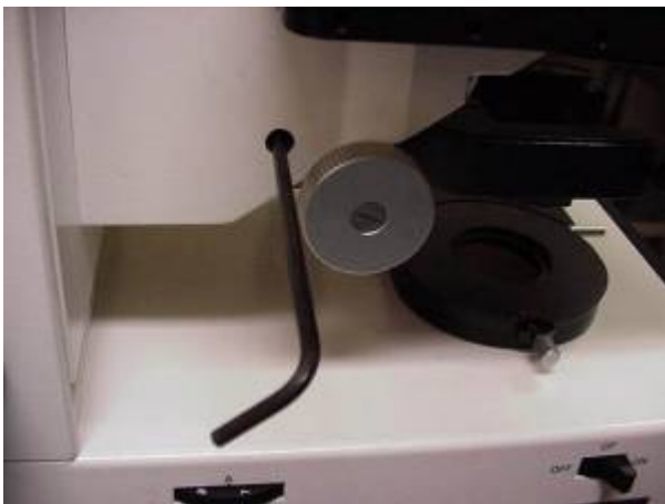
Figure # 1 Removing the condenser carrier
