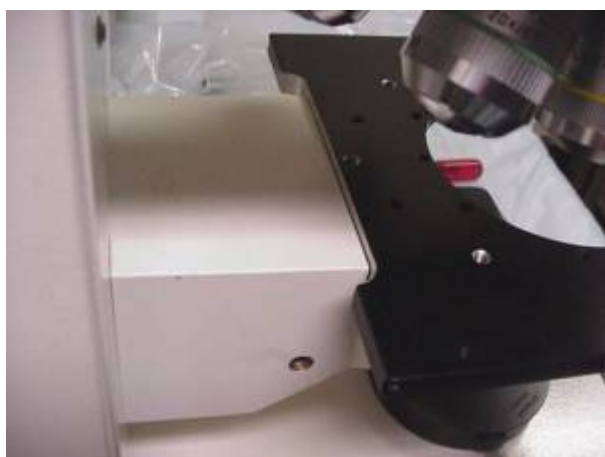
Figure 3 ASI stage mounted on carrier. Only the bottom plate is shown here for instructional purposes. The actual stage will have the middle & top plates installed.
