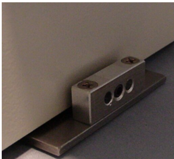
Figure 5. Clamp to tighten base plate to the microscope.
