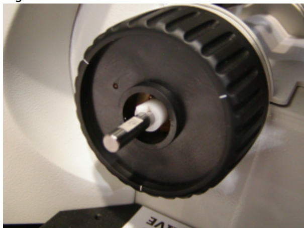
Figure 2: Pull knob straight off to expose shaft – Do not twist.
