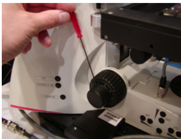
Figure 1: Use 1.5 mm Allen wrench to loosen setscrew to remove knob.
