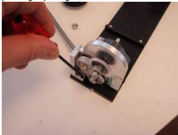
Figure 4. Remove the Z-drive assembly from the base plate by using the 7/64" Allen wrench to remove the horizontal adjustment screw.
