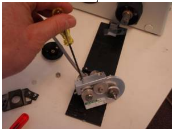
Figure 5. Use the 7/64" Allen wrench to loosen the two vertical adjustment screws.
