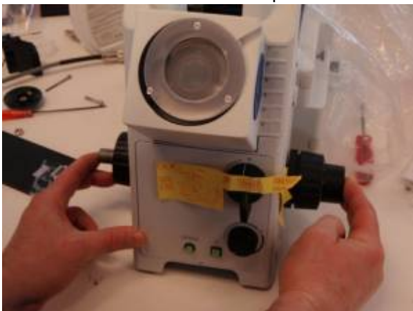
Figure 2. When installing coupler make certain that the right fine focus knob of the microscope is
