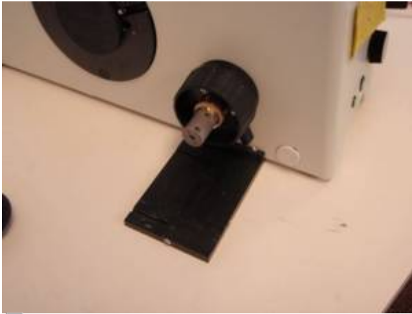
Figure 6. Slide the base plate assembly under the microscope as shown.
