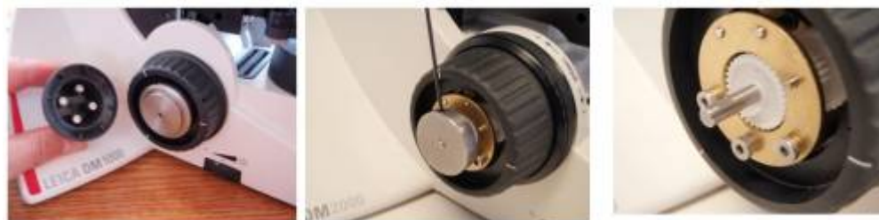
Figure 1: Use 1.5 mm Allen wrench to loosen setscrew to remove knob. Pull knob straight off to expose shaft – Do not twist.
