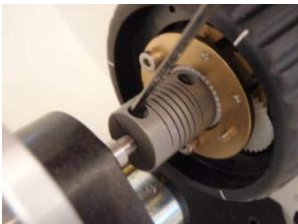
Figure 8: Use the 2 mm wrench to securely tighten the couple onto the fine focus shaft of the ASI Z
