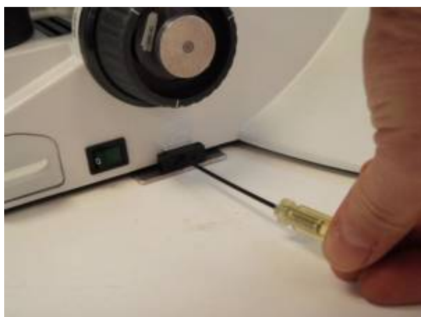
Figure 10: Tighten Baseplate set screw
