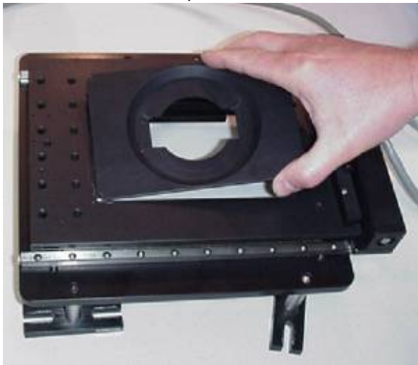
Figure 4: If you try to use the corner of the insert to compress both of the spring clips at once, it will be difficult to install the inserts.
