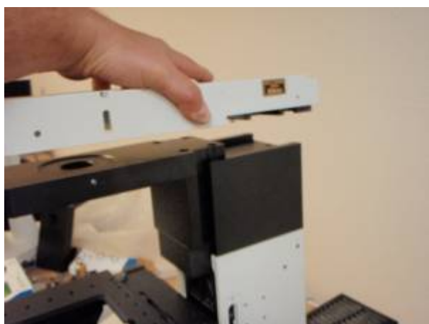
Figure 11a. Installing the trinocular mount back onto the microscope body
