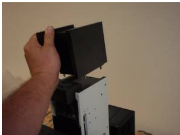
Figure 8. Installing the trinocular spacer, note alignment pins
