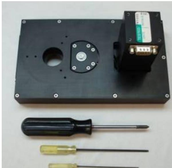
Step 2: Remove the nine 4-40 flat head Phillips screws from the case and remove the top cover. The cover should just clear the motor housing. On some older models, the cover will not clear the housing and the DB-9 connector may have to be removed with a 3/16" wrench first.
