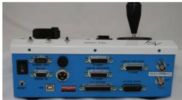
There is an option to control the Z focus with foot switches as well. If this option is requested the 9 pin serial out connector is used to connect the foot switches, and is labeled as such.
