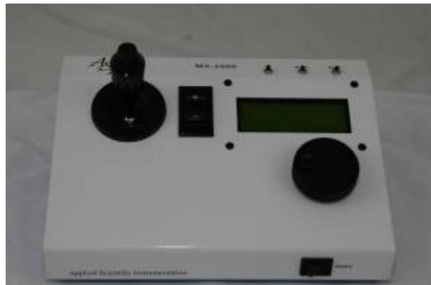
The toggle switch near the joystick provides for a rapid means of moving the stage up & down. Fine control of z position is accomplished with the Z focus knob, or by computer control.
