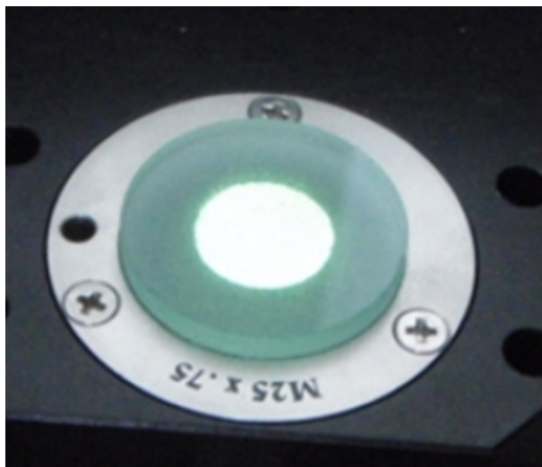
Figure 10: Light guide tip focused for Kohler
