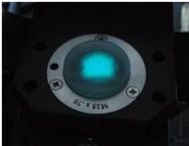
Figure 4a: Opening LED Aperture Overfills Objective
