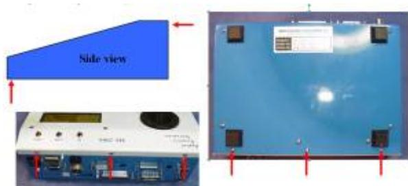
STEP 3: Remove the White Top lid from the Blue Case bottom. (Note: on older units a flat screwdriver may be required to pry the lid off by placing the screwdriver under the white lid at the corners on the top.)
