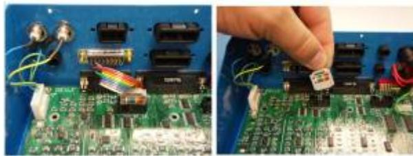
STEP 5: Using a 3/16" socket driver and pliers remove the two jack screw nuts and the two lock washers from the back of the Z-Linear Encoder Header. Remove any parts that fall inside the controller.
