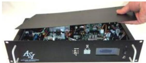
Second, remove the lid and set aside, as seen above. The Joypod header is located inside to the far right on the back of the rack mount. The header is screwed in the case with two 3/16" jack screws, or also two 3/16" jack screws with lock washers and nuts, or some units that have dual joypods have jackscrews on the right side and the left side both held in by two 3/16" jack screws.
