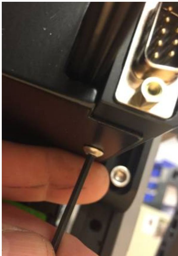
M4 cap screw removal bottom of slider.
