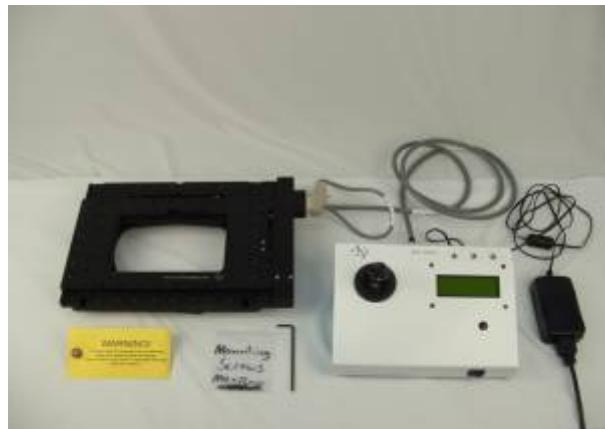
Remove System from packaging. Remove the stage locking bolt and connect stage controller with the provided cable. Connect the power brick to controller and turn on the system. Then, place the stage onto microscope stand.
