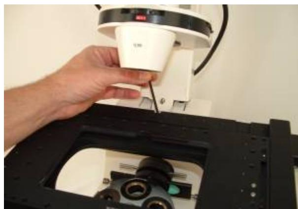
The stage will be shipped in the center position allowing you to install the rear mounting screw located at the back of the stage in the center position.
