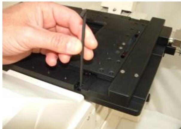
Next move the stage, again with the controller joystick, to the left until the plate cut out is aligned over the microscope mounting screw hole position. This will be near the leftmost position. Install the third mounting screw.
