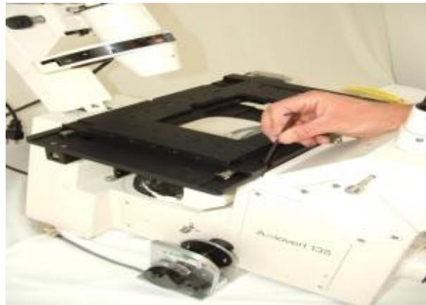
With the controller powered on move the stage, using the controller joystick, to the right until the plate cut out is aligned over the microscope mounting screw hole position. This will be near the rightmost position. Install the second mounting screw.
